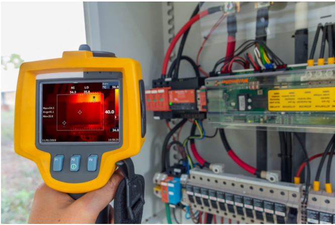
Fig. 6b: Industrial Condition Monitoring Using Thermal Imaging
