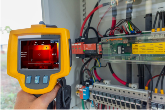
Fig. 6b: Industrial Condition Monitoring Using Thermal Imaging
