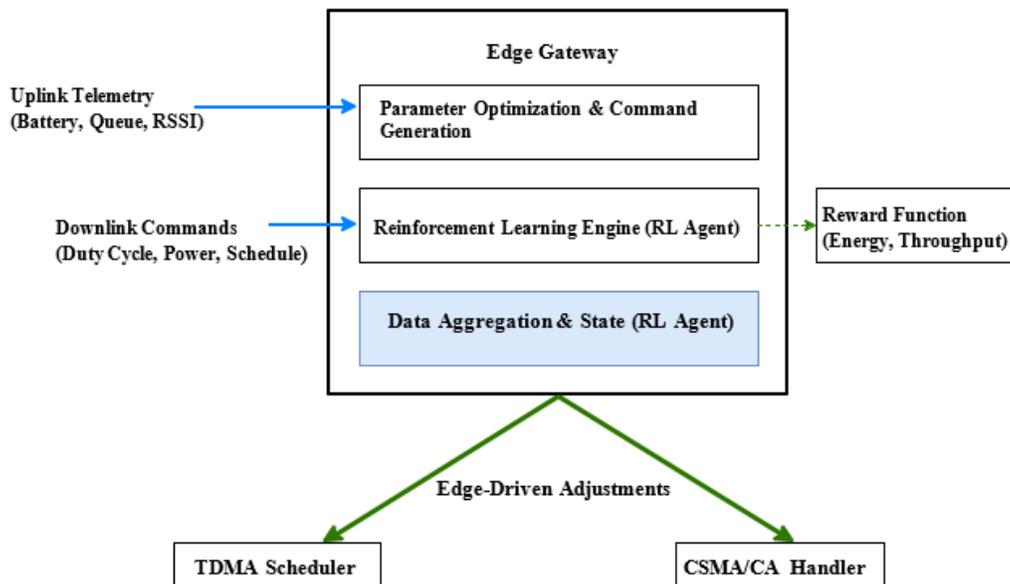
Fig. 1: Reinforcement Learning-Based Control Loop for Hybrid MAC Protocols at the Edge.
