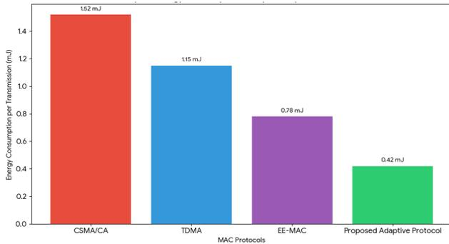
Fig. 2: Energy Consumption Comparison per Transmission.
