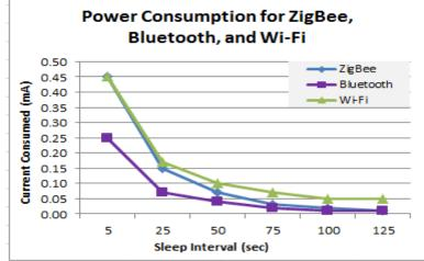
Figure 2. Power consumption for ZigBee, Bluetooth, and Wi-Fi [4]
