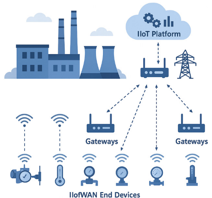
Fig. 1: LPWAN-enabled IIoT architecture with end devices, gateways, and cloud platform.
