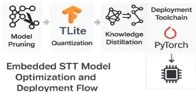
Fig. 5: Optimization and Deployment Workflow for Embedded Speech-to-Text (STT) Systems
